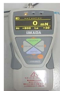
Fig. 3.2-1: IMADA ZTS-5N force gauge
